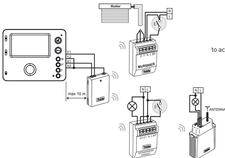
After suitably programming the Yokis devices, it will be possible: to activate the centralised closing of the rollers with a button (for example: ●●); a second button (for example: ●●●) will activate the turning off of the lights. For more information on **Yokis** products, please visit [www.yokis.com](http://www.yokis.com)
